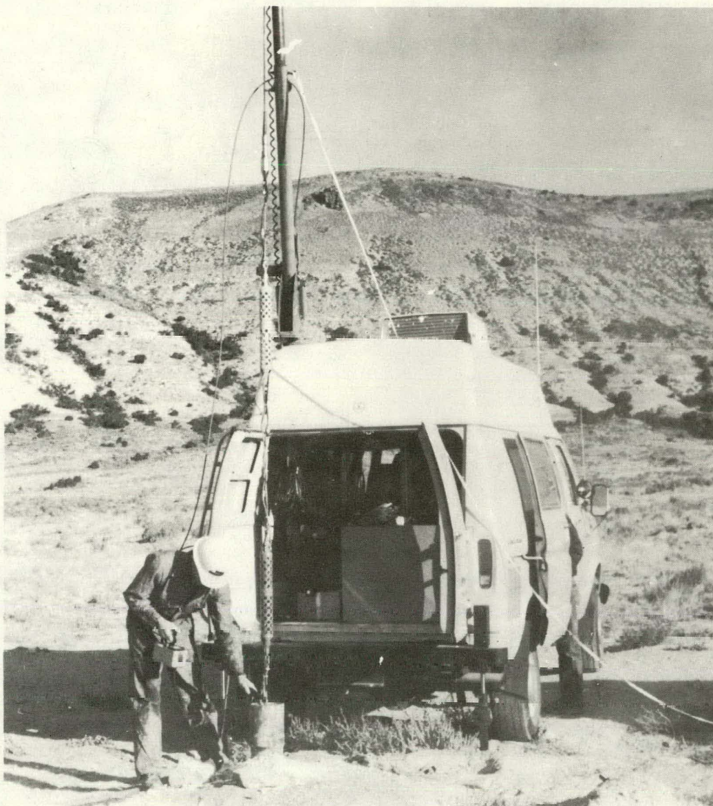
Figure 10. Mobile Field Support Unit Emplacing Downhole Equipment in Recovery Well
